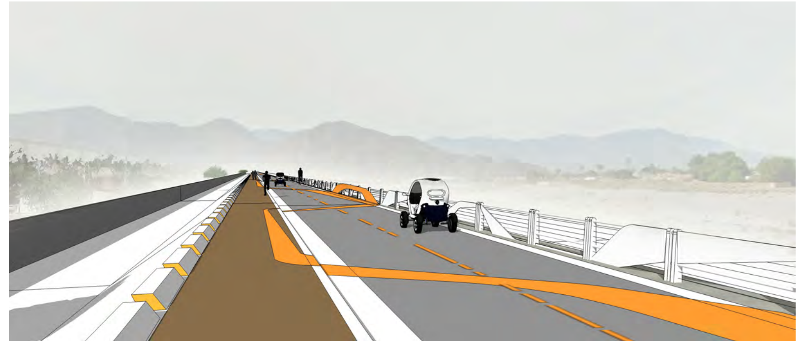
Situations with constrained levee width shall have curb-separated parallel paths.
